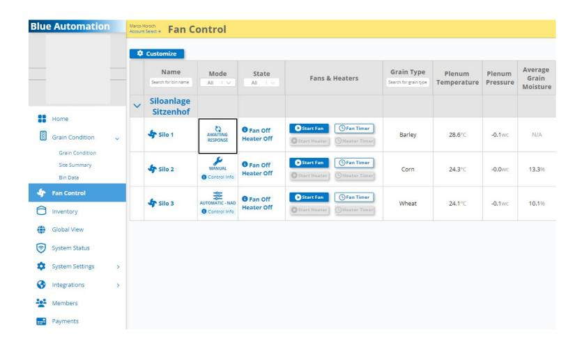
Step 9: The term "Awaiting Response" now appears in silo 1 under the "Mode" split, which indicates that the system is now processing your settings. Please refresh the page again after a minute. The split should now have the Automatic-Aeration mode applied
